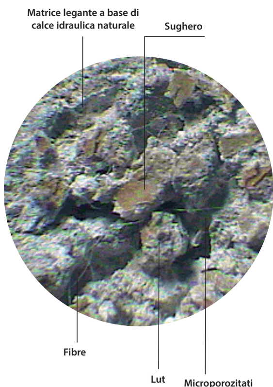
Diathonite Acoustix in sectiune (scara: 200%)
